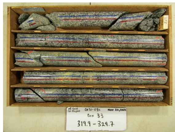
Figure 6.12: Localized weak potassic alteration with associated epidote veining
