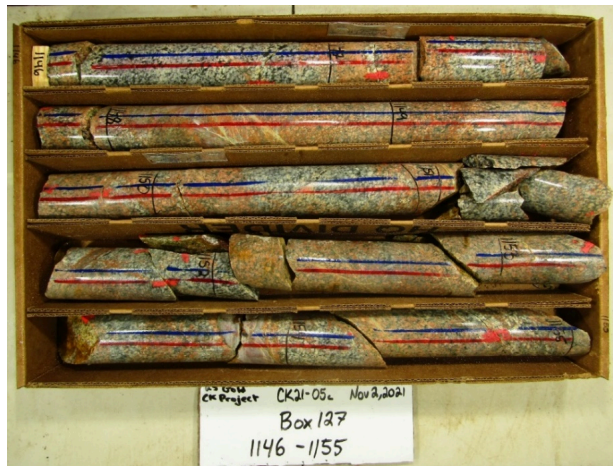
Figure 6.9: Moderate, localized potassic alteration in granodiorite
