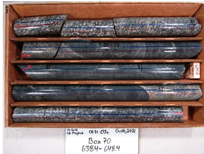
Figure 6.8: Typical mafic dike (center of photo) intruding granodiorite
