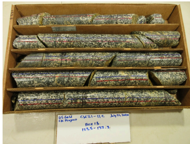
Figure 6.5: Relatively undeformed granodiorite
