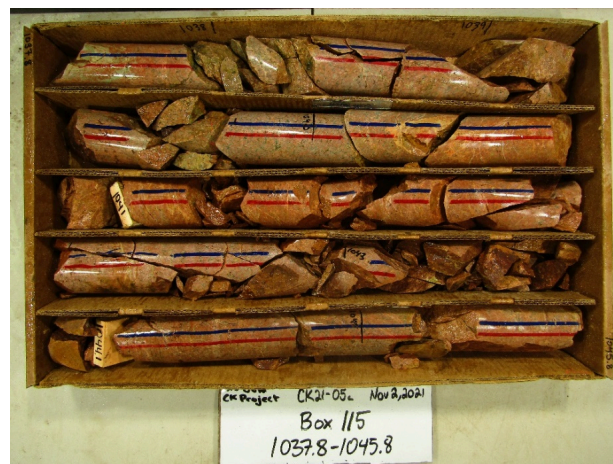
Figure 6.10: Intense, pervasive potassic alteration in granodiorite
