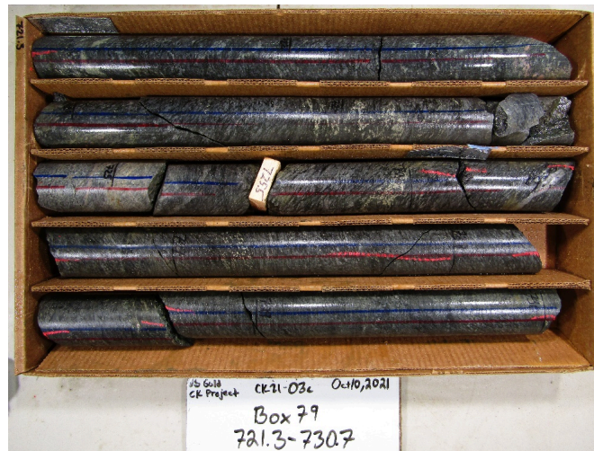
Figure 6.19: Pyrite +/- chalcopyrite aligned with mylonitic foliation
