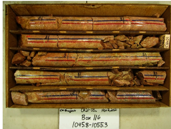
Figure 6.11: Intense potassic alteration with associated stockwork epidote veining
