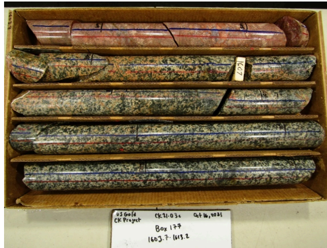
Figure 6.7: Felsic (pegmatite) dike (top row) within granodiorite
